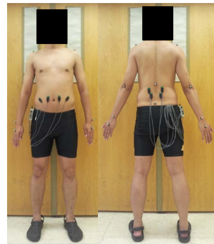
Figure 3. The placements of the Vicon reflective markers and EMG electrodes.
