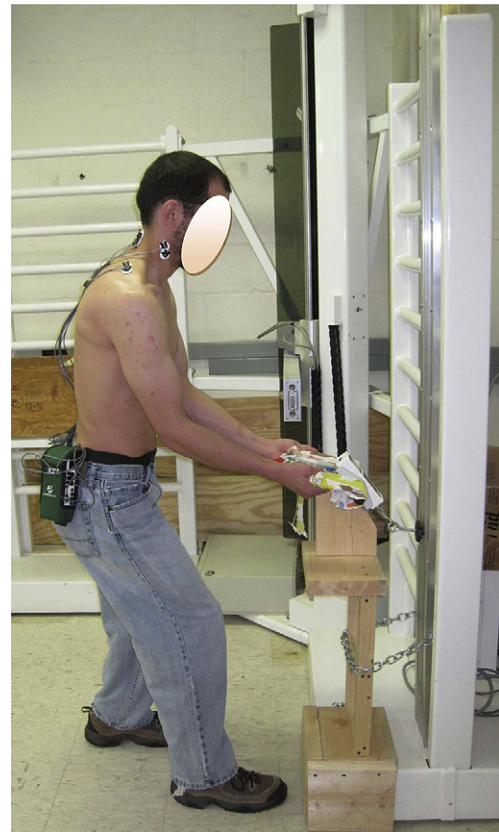
Fig. 2. A participant fitted with EMG surface electrodes performing isometric pulling task using the custom-built strength testing device.
