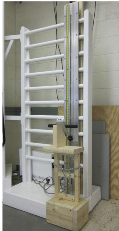
Fig. 1. Picture of custom-built isometric pulling strength testing device used in this study to induce physical demand.
