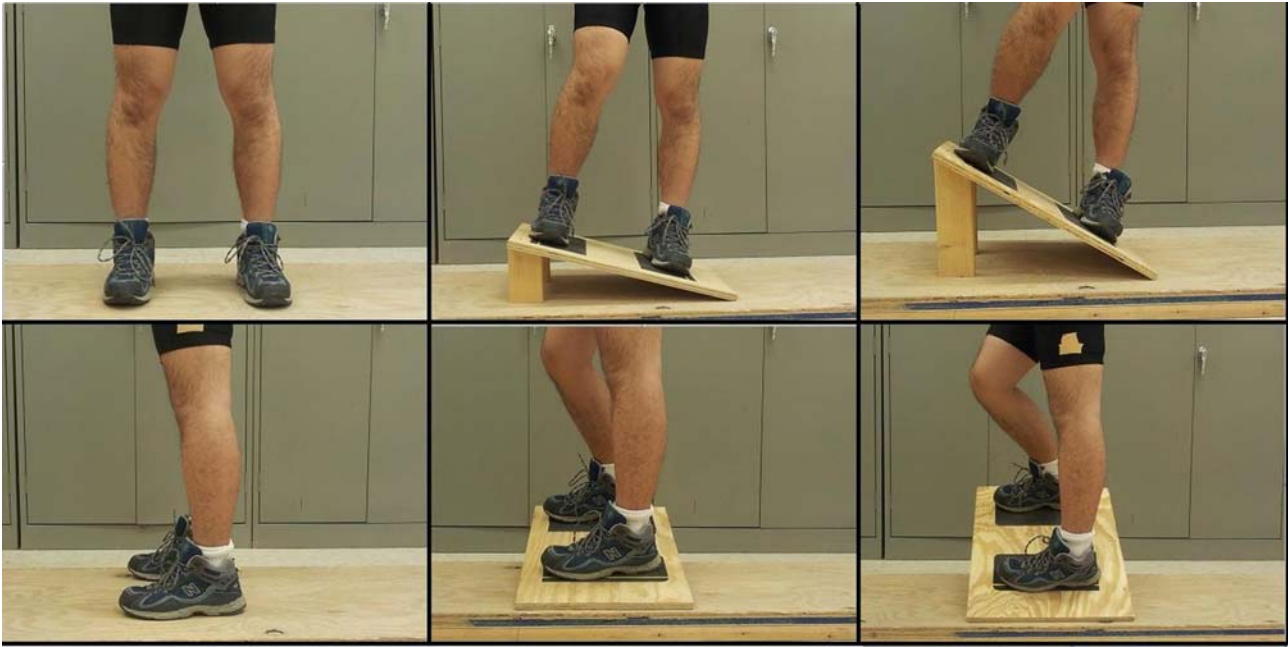
Figure 1. Frontal and side views of the ground conditions (left panel, flat; centre panel, 15° slanted; right panel, 30° slanted).
