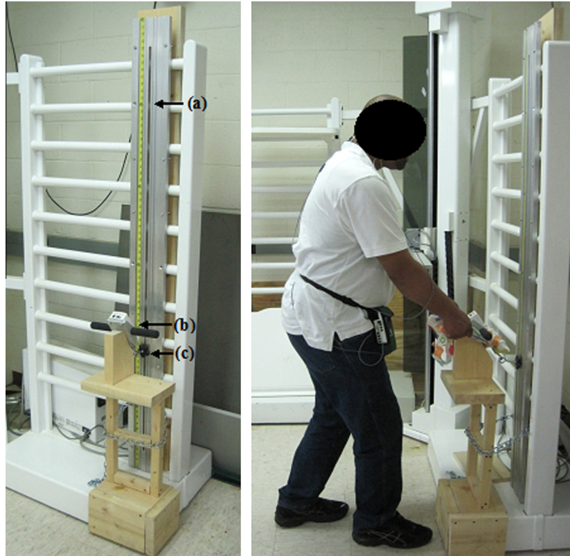
Fig. 1. (a) Picture of the pulling exertion device and (b) a participant performing isometric pulling task simulating force exertion during bed-to-stretcher patient transfer task.
