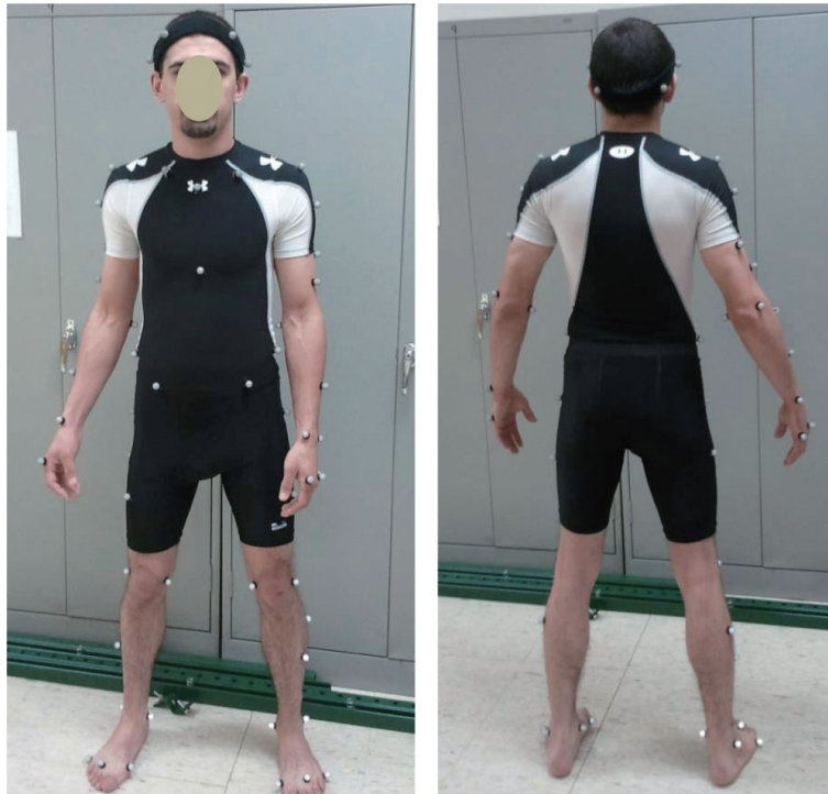
Fig. 2. Subject in the full custom set of 62 retro-reflective markers. (Colours are visible in the online version of the article; http://dx.doi.org/10.3233/OER-140213 )
