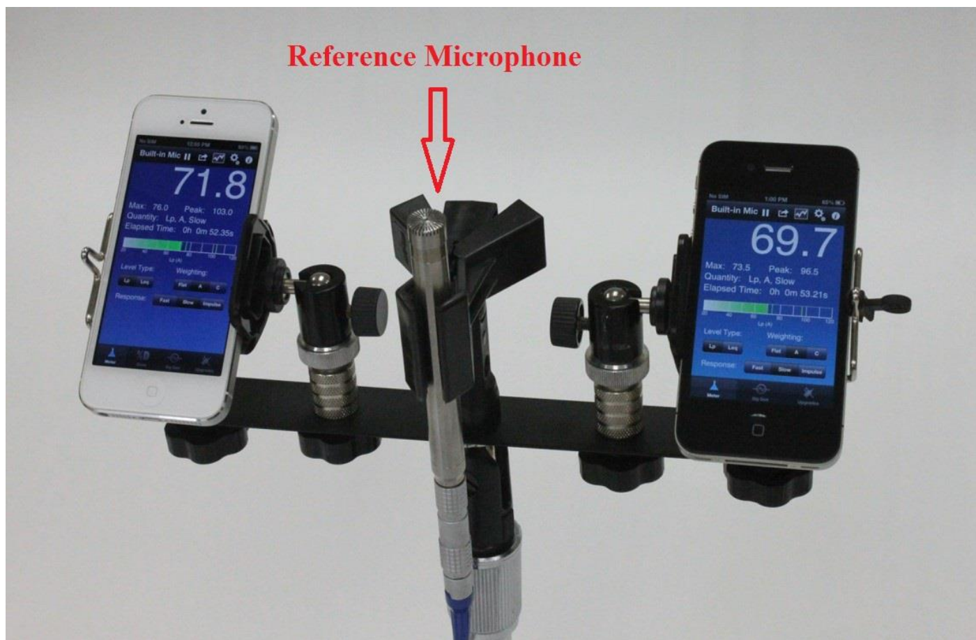
Figure 1. Testing the SoundMeter app on the iPhone 5 and iPhone 4S against a 1/2" Larson-Davis 2559 random incidence reference microphone
