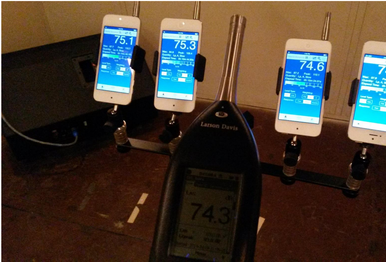
Figure 3. Laboratory testing of 4 iOS devices using MicW i436 and comparing the measurements to a Larson-Davis type 831 sound level meter (pink noise at 75 dBA)
