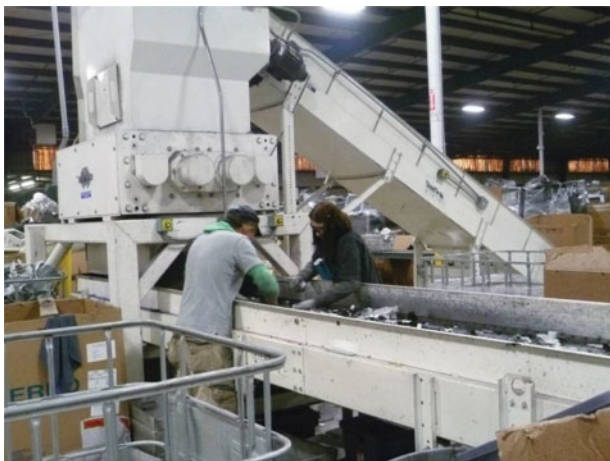
Figure 2. Sorters removing non-plastic and non-metal pieces (i.e., rubber pieces), green board pieces, and copper at the shredding machine.
