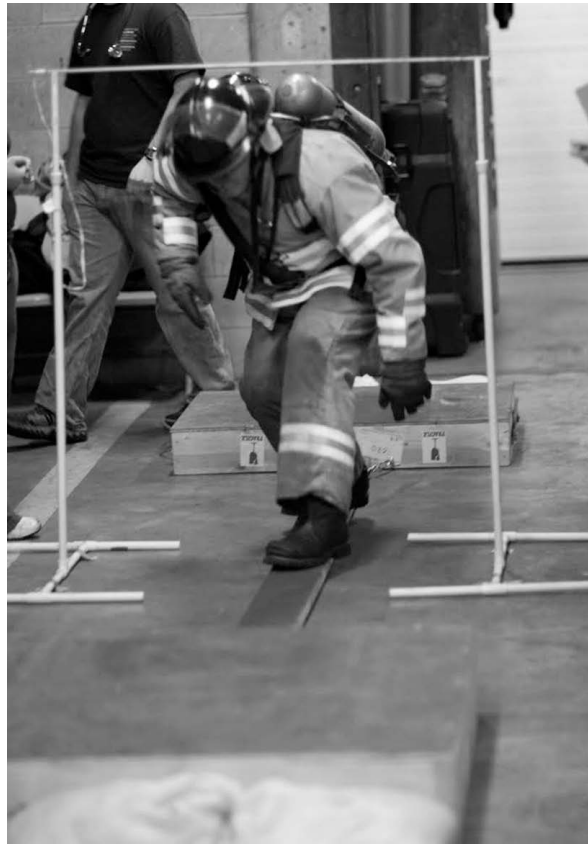
FIGURE 21.3 Test of overhead obstacle clearance while wearing protective clothing and breathing apparatus.
