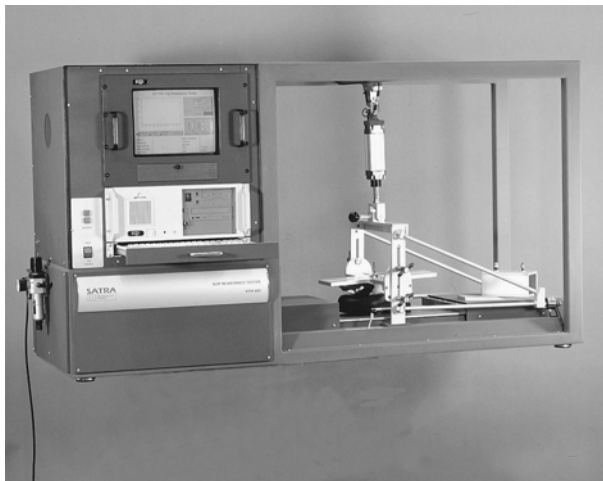
FIGURE 12.5 Slip resistance tester STM603. (From Chang, W.R. et al., Ergonomics , 44, 1233–1261, 2001.)
