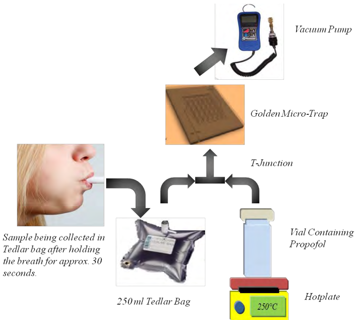
Figure 2.3 Experimental setup for the adsorption phase with arrows showing the direction of the sample flow.
