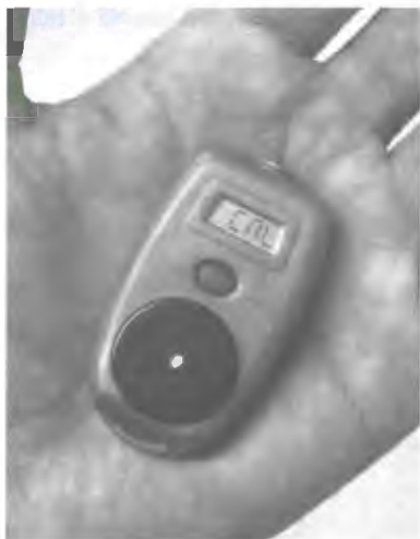
Figure 1.41. KWJ pocket instrument with incorporated electrochemical sensor for either CO, H 2 S, H 2 , or ozone. The instrument continuously displays real-time concentration and can report dosimetry information including the 8-h time-weighted average concentration, the total exposure (ppm h), and the magnitude and time of occurrence of the maximum. (Reprinted with permission from Ebeling et al. 2009. Copyright 2009 Elsevier.)
