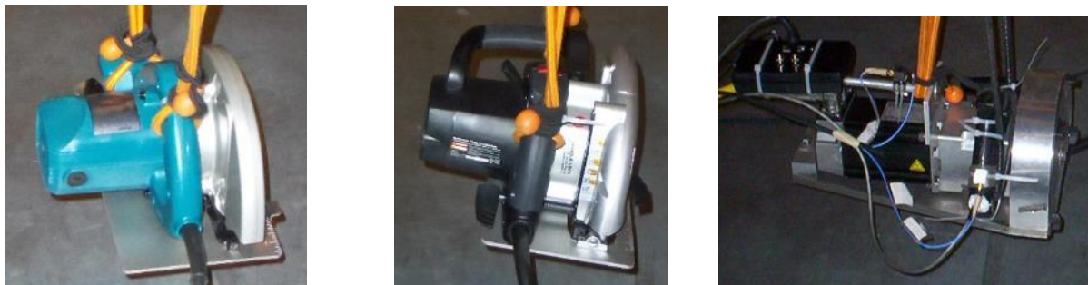
Figure 6: Side view of the Makita, Craftsman, and Research circular saws respectively from left to right.
