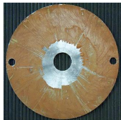
Figure 4: On the left, front view of the blade stiffener without any treatment. On the right, front view of the blade stiffener with room temperature vulcanizing silicone treatment, which acts as a viscoelastic damping treatment.
