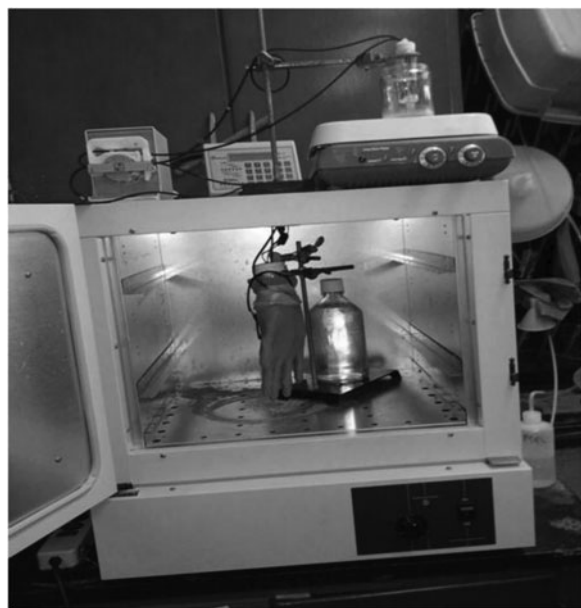
Figure 2. Photograph of the whole-glove permeation set-up showing from the top left of the opened incubator the peristaltic pump, the microprocessor (center top) to control the clenching of the double-gloved robot hand (incubator center, held by a clamp, but with cyclohexanol container that the hand dips into absent for clarity), with the clamped sampling point on top of the incubator right side standing on its magnetic stirrer-hotplate and connected to the hand and peristaltic pump with black Viton tubing. A multi-strip is at the bottom left. The vent to the nearby fumehood from the center of the top of the incubator is also not shown for clarity.
