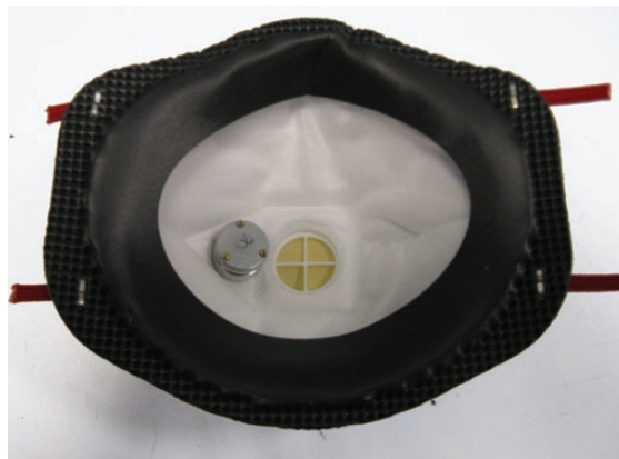
Figure 2 A miniature sampler fitted to a filtering facepiece (FFP 3) mask
