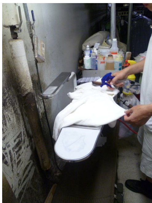
FIGURE 3. Employee spraying shirts with a solution containing SolvonK4™ to pretreat fabrics before drycleaning cycle.
