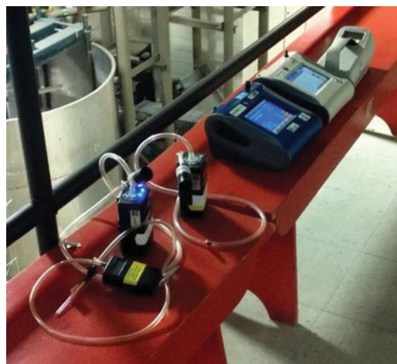
Figure 2. Background sampling with three real time data logging particle counters (condensation particle counter and optical particle counters), two 25 mm open-face filter cassettes, and one sorbent tube (for a process solvent).
