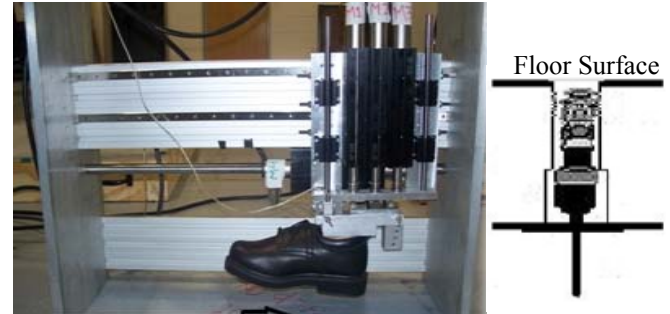
Fig. 2: Slip-testing apparatus (left) and fluid pressure sensor that is embedded in the floor (right).
