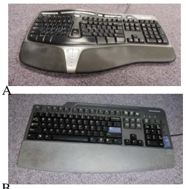
Figure 1 – Study keyboards: A = fixed split-angle; B = standard
