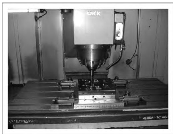
FIGURE 1. Machining operation to manufacture a mold to be used in plastic injection. Metal working fluids (MWFs) will be sprayed on the tool and the metal being machined. The MWF runoff and metal shavings will be collected in a large container located under the machine.
