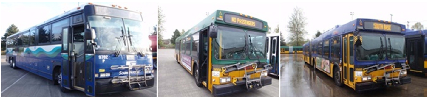
Figure 1 - high-floor coach bus (left), low-floor coach bus (middle), and low-floor articulating bus (right)
