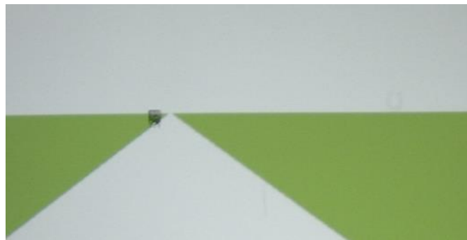
FIGURE 1 Portion of a projected scene showing the LED to the left of the roadway simulating a service vehicle.
