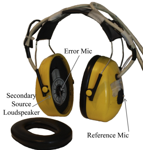
Fig. 3. Active hearing protector physical model demonstrating placement of active sensing and control elements.
