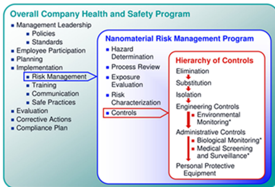
Fig. 5 Components of an overall health and safety program that includes nanomaterial risk management (Schulte et al. 2008a, b)
