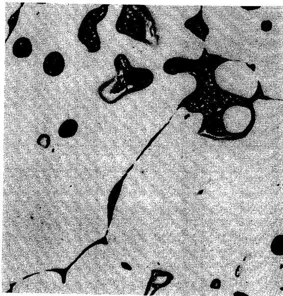
FIGURE 12. - Microstructure for Magnesium-Reduced Molybdenum From Run MoA 38 (500X). Etchant, K_3Fe(CN)_6-KOH-H_2O . Many oxide inclusions.
