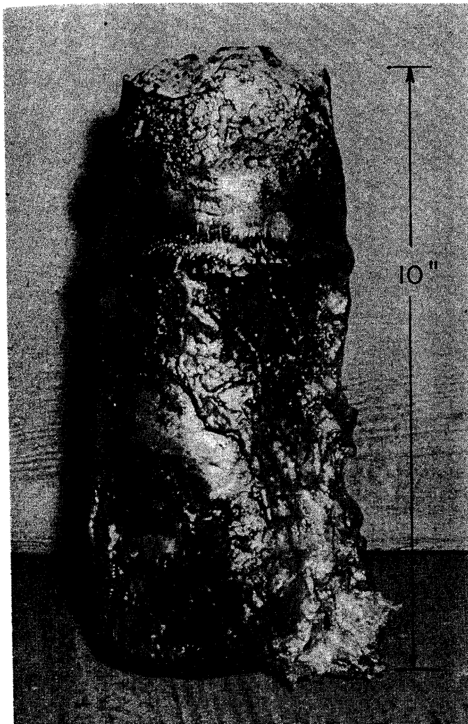
FIGURE 5. - Thirty-Seven-Pound Cast Molybdenum Regulus.
