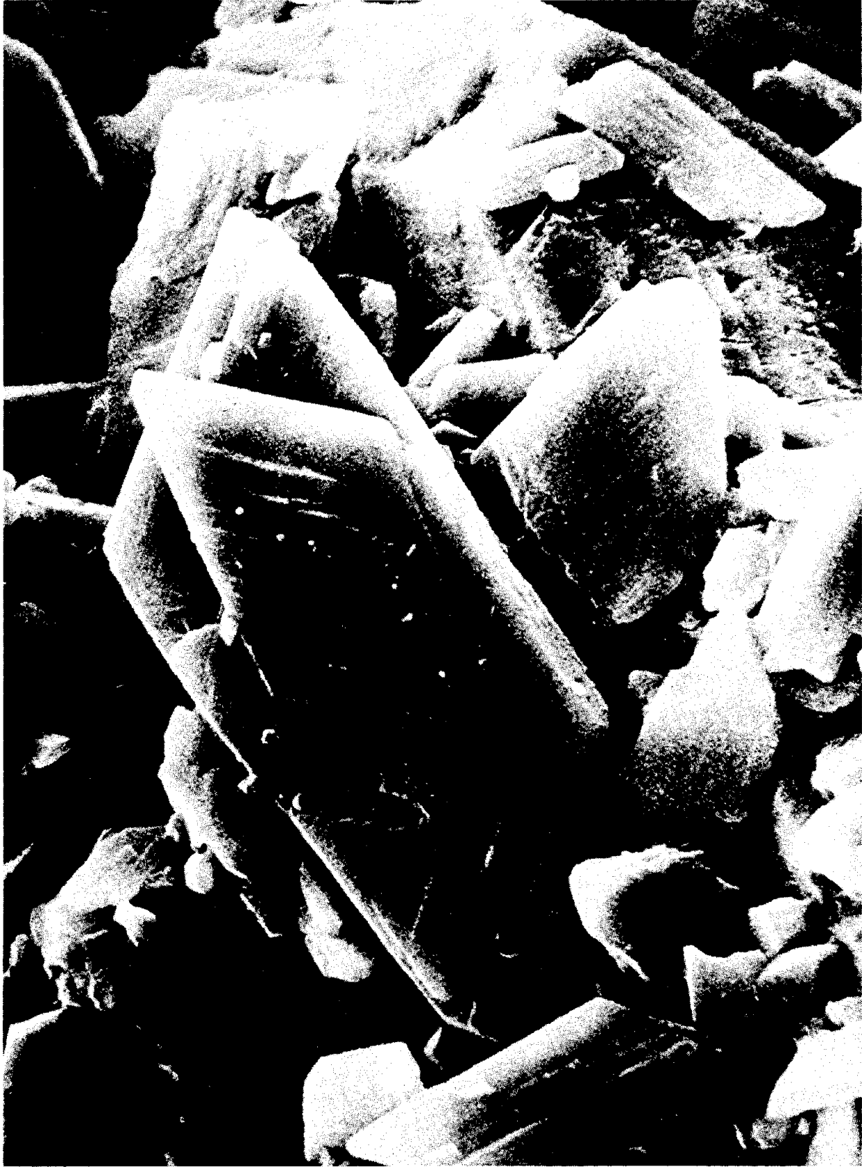
FIGURE 2. - Scanning electron microphotograph of phosphogypsum (X 1,000).
