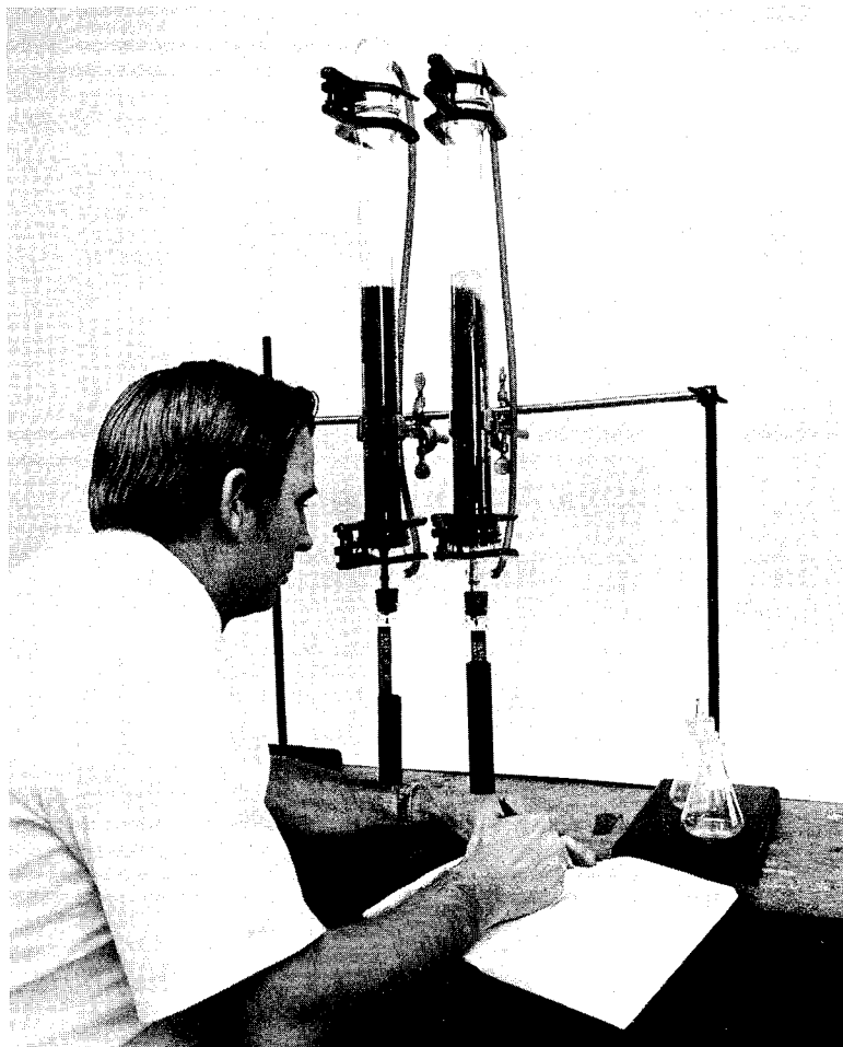
FIGURE 3. - Sand column test apparatus.
