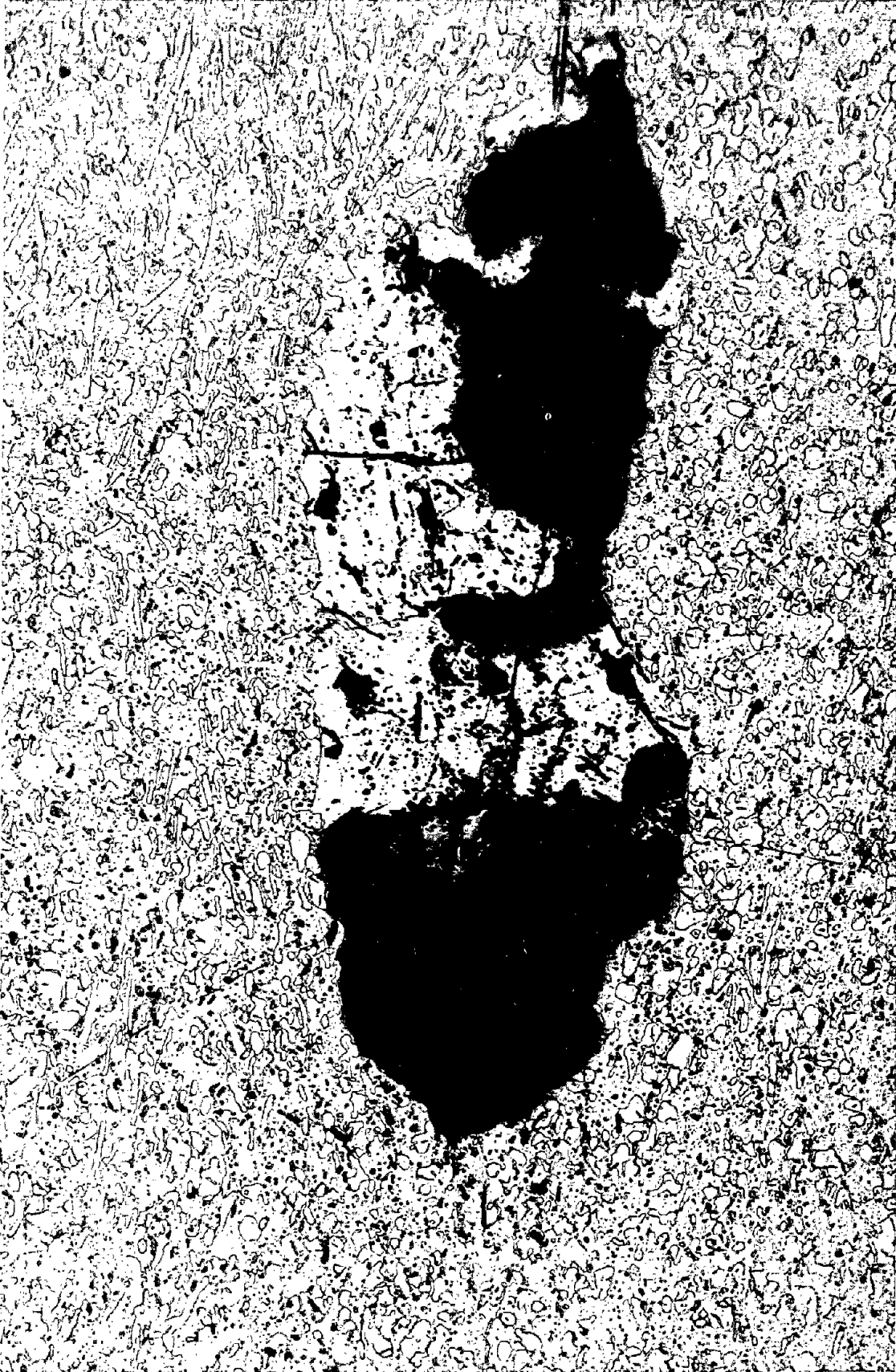
FIGURE 16. - Typical nitride inclusion found in plate made from sponge contaminated by diffuse air leak during distillation, X 50.
