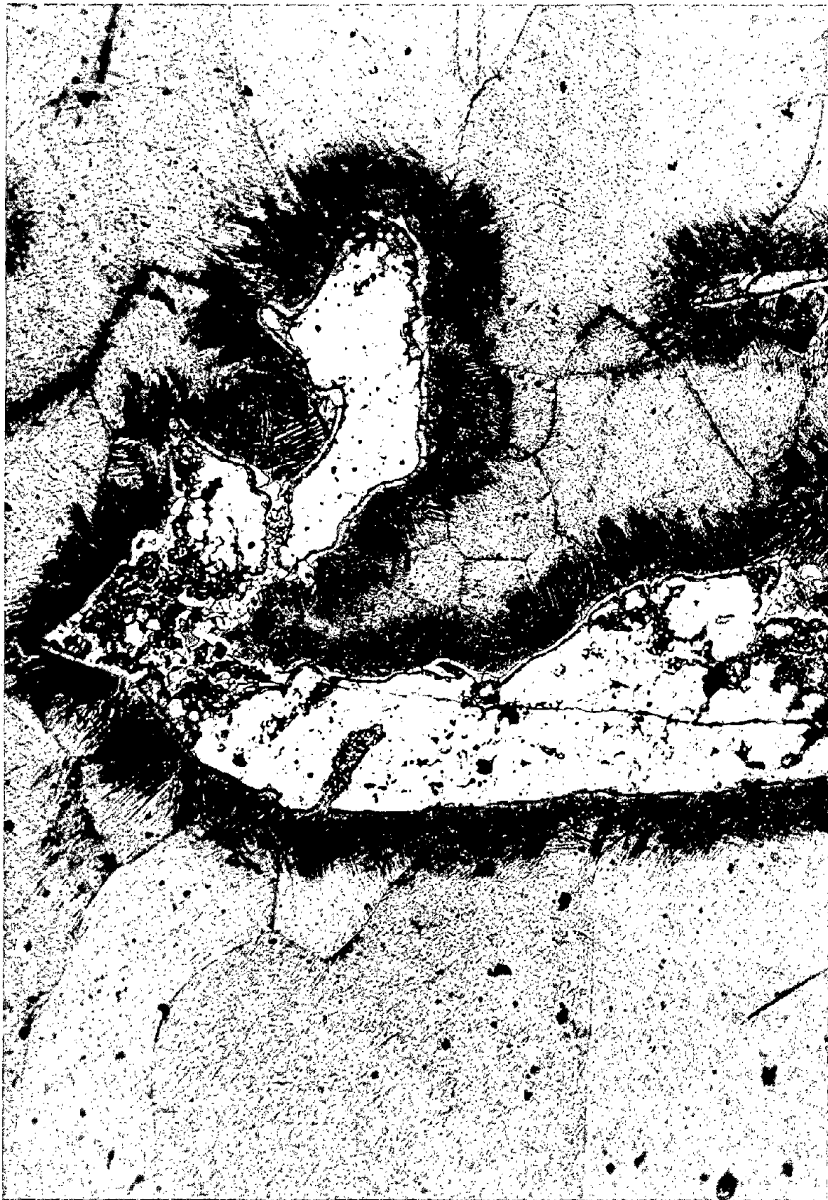
FIGURE 22. - Photomicrograph of TiN fragment after 60 seconds in molten titanium, X 50.
