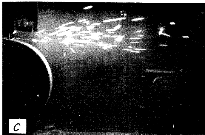
FIGURE 2. - Spark showers from elemental metals. A , Titanium; B , chromium; C , zirconium; D , vanadium.
