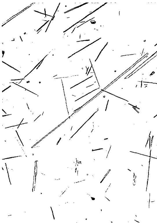
FIGURE 17. - Photomicrograph of particles from Wiley-milled asbestos 2.
