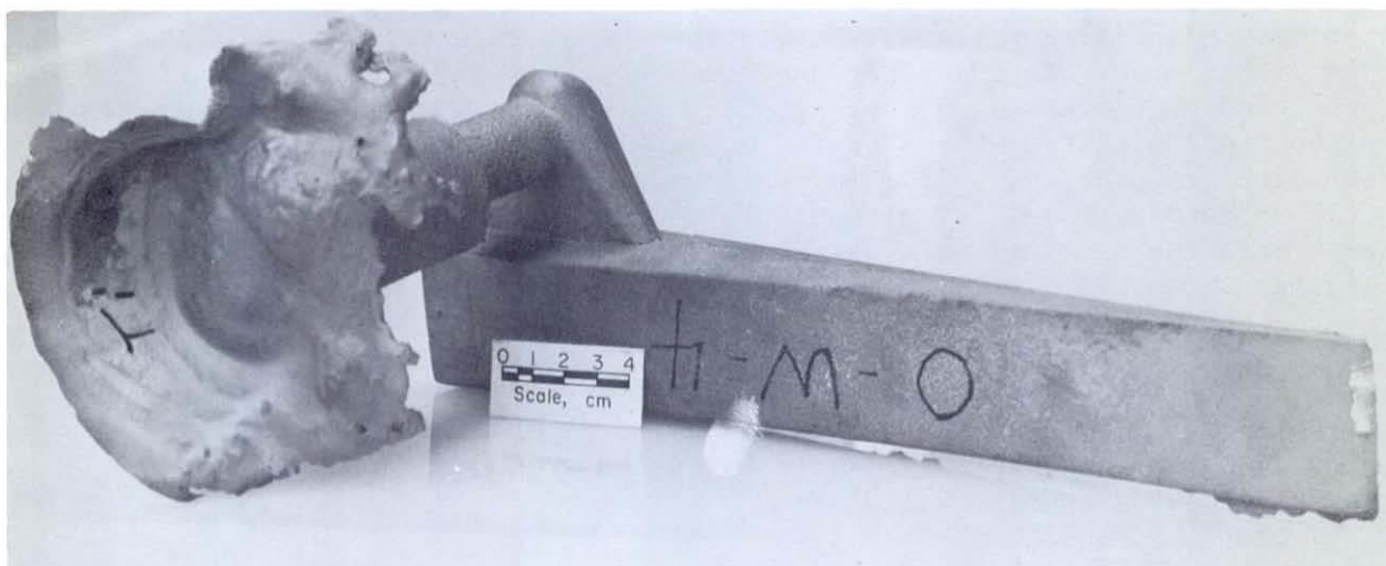
FIGURE 5. - Typical inductoslag cast wedge poured in an unwashed olivine mold.
