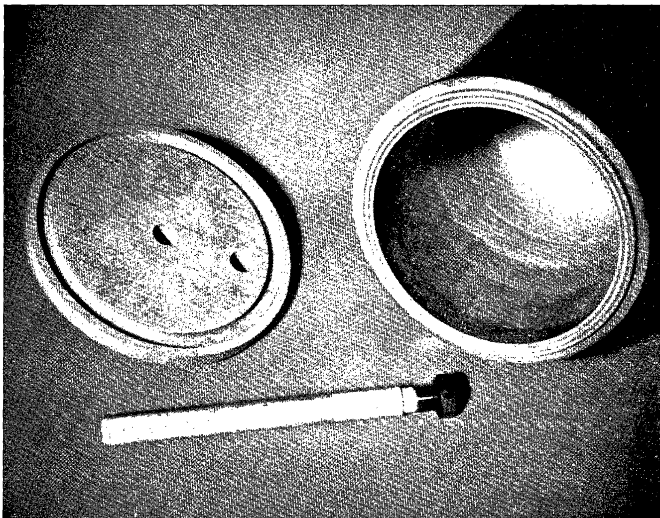
FIGURE 7.— One-liter pressure vessel, top and lid after electrodeposition of platinum coating.
