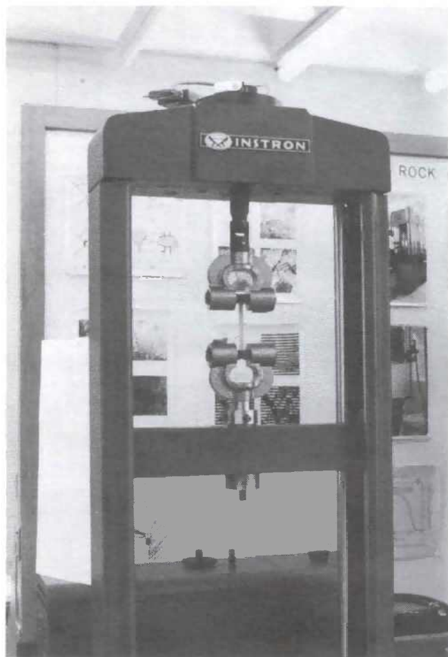
FIGURE A-1. - Instron TM 100-kg universal testing machine with test specimen.
