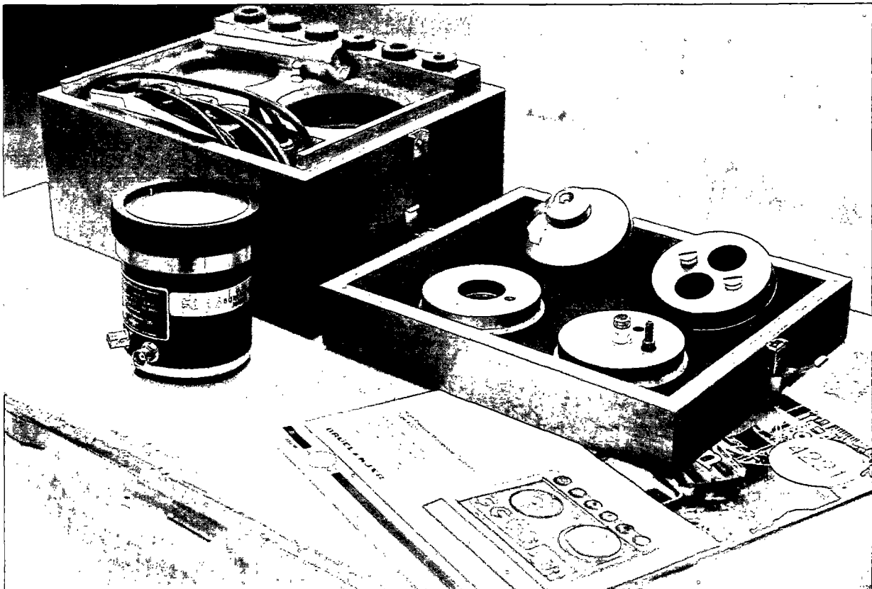
FIGURE 13. - High-pressure, low-frequency calibrator.
