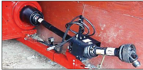
1: Driveline shield is in place, in good condition, and rotates easily.
