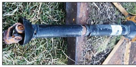
3: Driveline shield is in place but is bent, cracked, sliced, and/or does not rotate.
