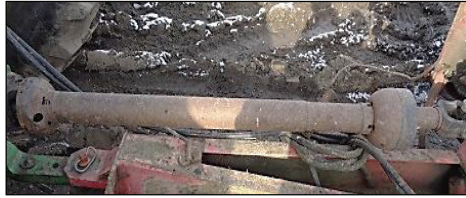
4: Driveline shield is in place but is bent, cracked, sliced, and/or bearing is missing or damaged.
