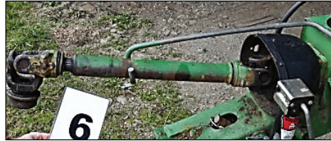
5: Driveline shield is missing, or the machine never had a driveline shield.
