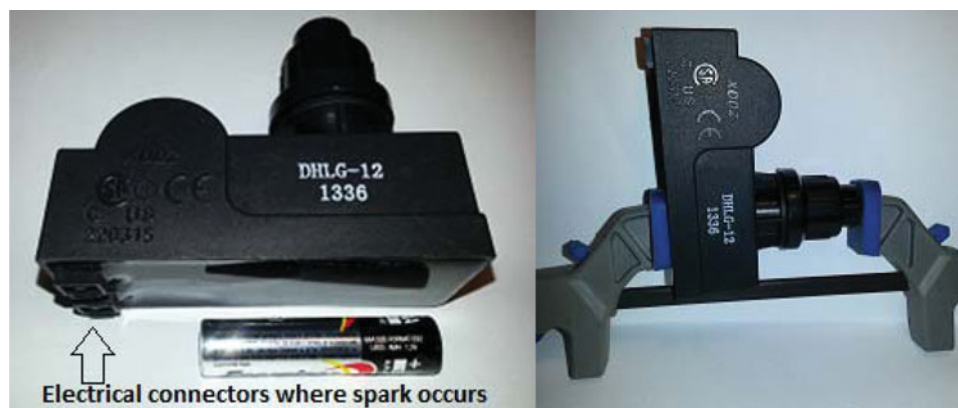
FIGURE 1. Gas grille igniter
