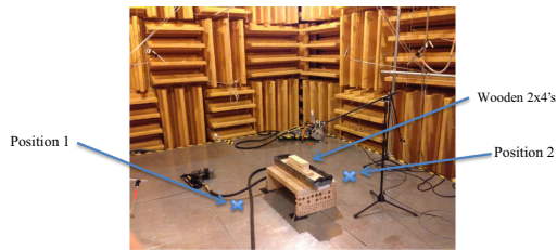
Fig. 4—Framing nailer test setup. Wooden two-2 × 4s are stacked in the sand box to receive the nails. The framing nailer operator made approximately ten measurements in position 1 and ten measurements in position 2.
