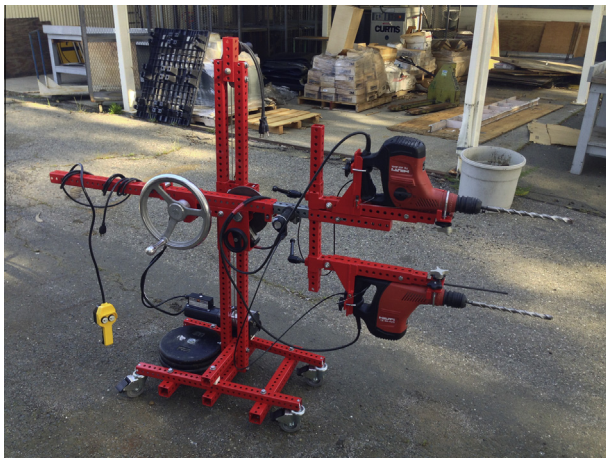
Fig. 3. Final design of universal drilling that can drill 2 holes simultaneously into concrete. Drills are supported in saddles that are attached to a T-bar mounted to the end of the barrel. Turning the round aluminum handle advances the activated drills into concrete. The small black round handle locks the barrel at the desired angle. The barrel is raised and lowered on the vertical columns with an electric winch.
