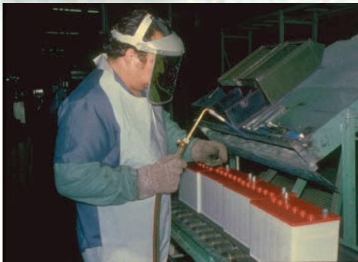
Auto battery manufacturing with lead exposure ventilation hood protection. (Visalia, Calif., 1983)
