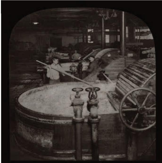
Operators of paper mill pulp beaters have no eye protection from chlorine used in paper bleaching. (Keystone View Co.)
