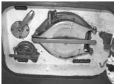
Fig. 2. Waste port and controls.
