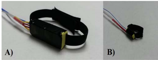
Figure 1 Adapters for measurement of vibration and force at the A) palm and the B) finger
