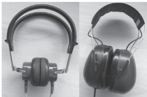
Figure 1. Supra-aural and circumaural earphones. A photograph of a supra-aural (Telephonics TDH-39P) earphone is shown on the left. A circumaural (Sennheiser HDA200) earphone is shown on the right. The supra-aural earphone enclosure rests on the listener's pinna during testing. The cushion on the circumaural earphone enclosure forms a seal around the periphery of the pinna but does not rest on the pinna during testing.
