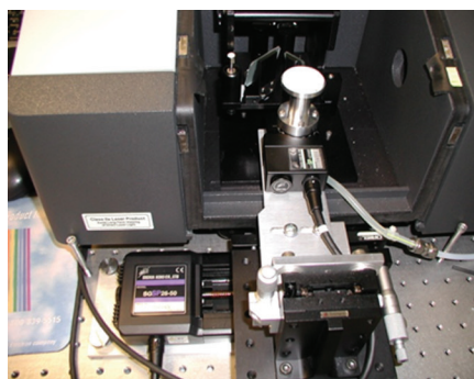
Figure 1 Picture of the motorized stage in the diffuse reflection unit inside the FT-IR spectrometer and a schematic of the diffuse reflection process (from Chirila et al., 2011 ).
