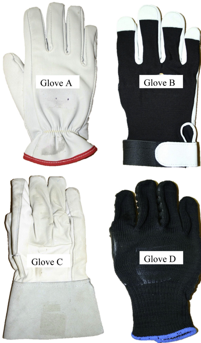
Fig. 1. The gloves used in the study and their major vibration isolation materials: Glove A – thick gel pad; Glove B – cellular air bubbles; Glove C – air bladder with pump; and Glove D – dipped neoprene.
