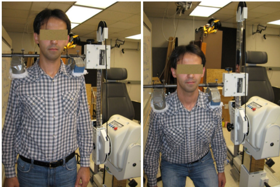
FIGURE 3. Customized Biodesign attachment for measurement of maximum voluntary exertions.
