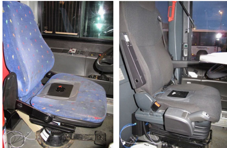
Figure 1. Examples of mechanical pedestal seat (left) and air-suspension seat (right). The seat pad accelerometer was rigidly taped to the seats.
