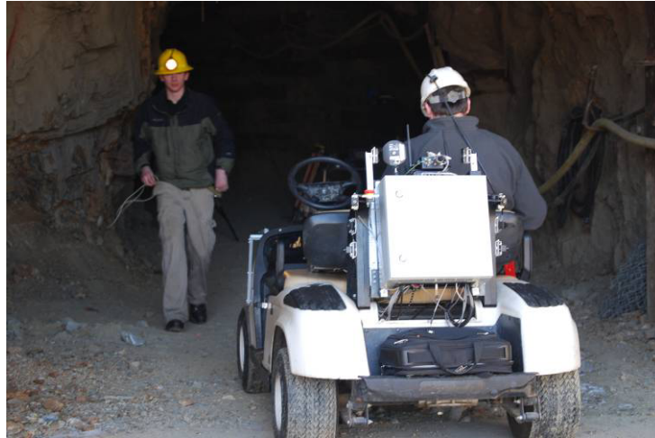
Figure 3: EZ-Go AMR in the Colorado School of Mines' Edgar Mine.
