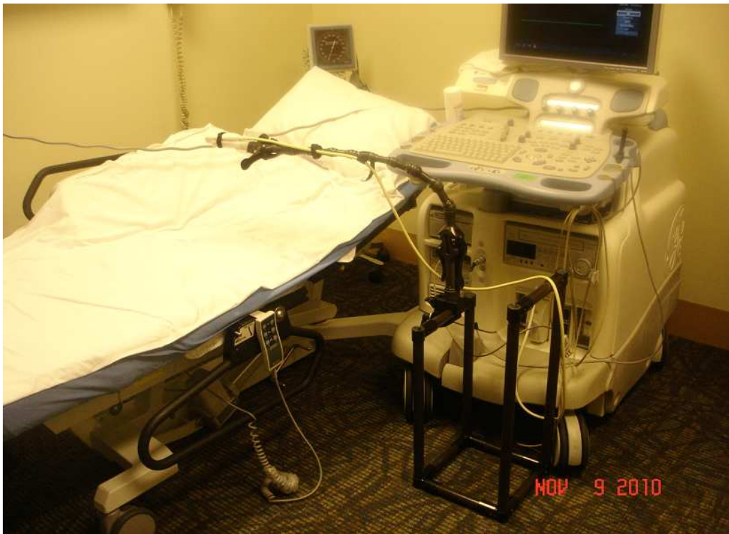
Figure 3.19. The functional prototype consisting of a probe holder, articulating arm, and a mounting stand.
