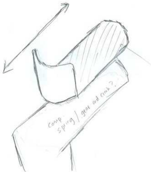
Figure A.18. This is an elbow augmentation system, which pushes the sonographer's elbow towards the patient. The idea was that an external force to the back of the elbow would provide the sonographer augmentation to pushing activities.
