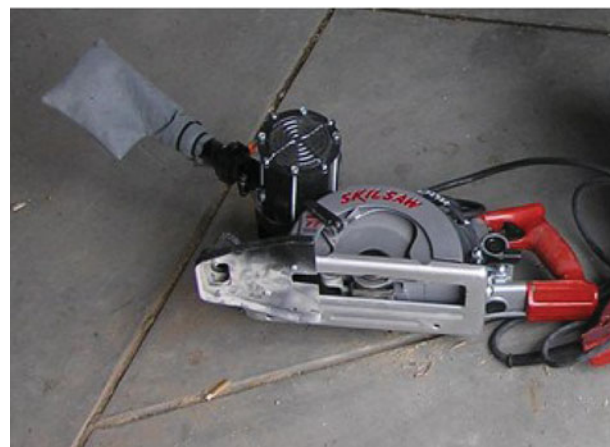
FIGURE 3. Circular saw with aftermarket local exhaust ventilation. (color figure available online)
