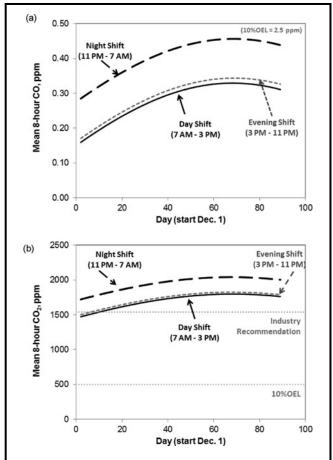
**FIGURE 2**. Eight-hour time-weighted averages of (a) CO and (b)  $CO_2$  by shift over the 90-day simulation period for baseline simulations (2 heaters and 2 pit fans).
