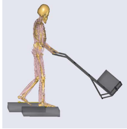
Figure 2: Graphical representation of the musculoskeletal model developed using AnyBody modeling system to model the cart pushing exertions
