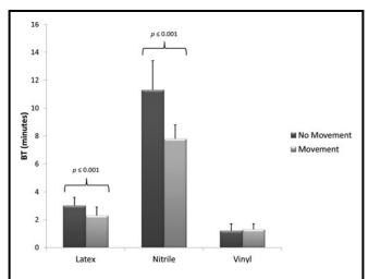
**FIGURE 1.** Breakthrough time (BT) for different glove types, no movement versus movement. Significant reductions in BT are shown with brackets. Significant decreases in BT were observed with the latex and nitrile gloves.
