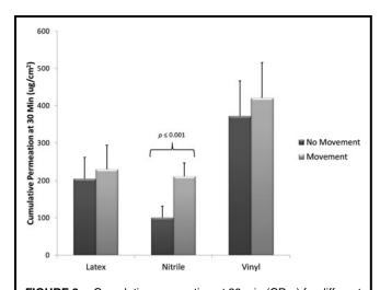
**FIGURE 3**. Cumulative permeation at 30 min ( $CP_{30}$ ) for different glove types, no movement versus movement. Significant increases in  $CP_{30}$  are shown with brackets. A significant increase in  $CP_{30}$  was only observed with the nitrile glove.
