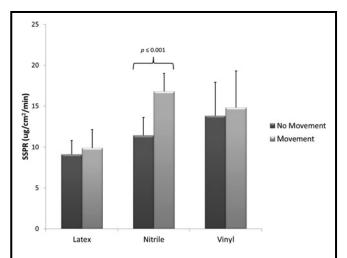
**FIGURE 2**. Steady-state permeation rate (SSPR) for different glove types, no movement versus movement. Significant increases in SSPR are shown with brackets. A significant increase in SSPR was only observed with the nitrile glove.
